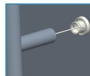
After ensuring there are no obstructions behind the wall,drill a 1/2-in hole through the drywall at the wall marking made earlier. Inset the **Wall Bushing ⑩** through the **Power Wall Flange ⑪** and screw the bushing into the hole you drilled into the drywall.Screw the bushing until it's snug and the small holes in bushing are aligned vertically.
