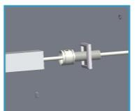
After ensuring there are no obstructions behind the wall, drill a 1/2-in hole through the drywall at the wall marking made earlier. Inset the **Wall Bushing ⑩** through the **Power Wall Flange ⑪** and screw the bushing into the hole you drilled into the drywall. Screw the bushing until it's snug and the small holes in bushing are aligned vertically.
