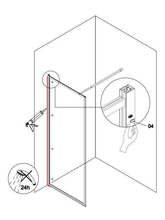
Before the final set up of this shower enclosure, check its watertightness. In case of leakage, retighten the screws and if necessary add silicone.
