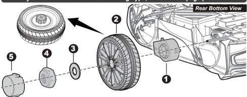
Remove all the parts from the rear axle.
