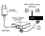
Ensure that the smart phone is within the same WIFI network of the device to ensure an effective connection between the smartphone and the device.
