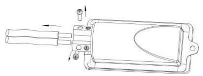
4. Replace the light with a new one and re-assemble.
