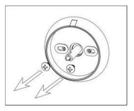
3. Take off the unit and loosen the LED cable connections carefully.
