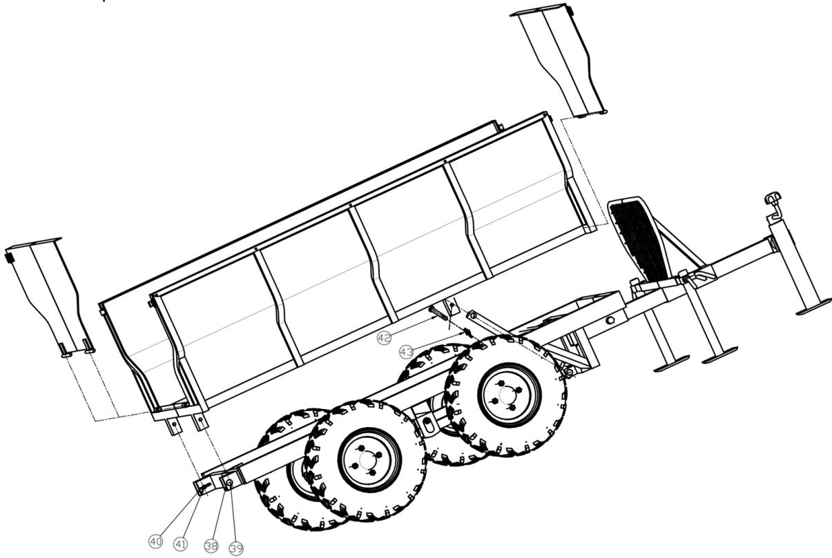
4. Install the fence, using 6-M8\*30 bolt, M8 nut, fasten the fence. **SEE FIGURE 4.**
