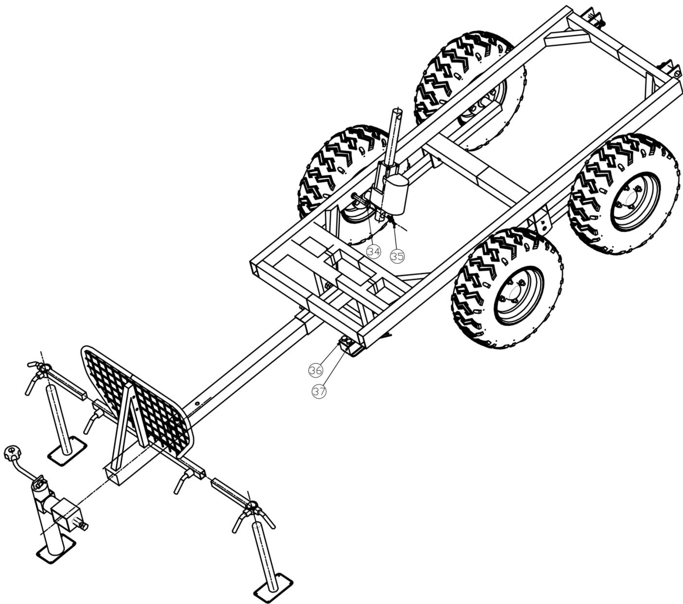
3. Install the box, using 2- M18\*80 pin roll, 2-"R" pin,2-M16 nut, Install the linear, using 12\* 70 bolt M12 nut with the box. Install the door panel and fasten it. **SEE FIGURE 3.**
