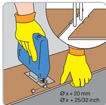
If you have heating pipes, measure their exact position and mark it on the laminate.
