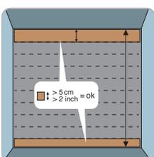
Measure the length of the room from the point where you plan to start to the wall where you will end. Divide this by the width of a plank. The purpose is to never end with a plank that is less than 5cm wide. If that is the case, you should modify the width of the first row (saw the plank so that you don't start with a full plank, but it should be more than 5cm).
