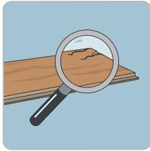
Check all planks for visible defects in optimal light conditions, both before and during installation. Planks with defects must not be used.
