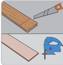
If using a hand saw, cut on the pattern side, if using an electrical jigsaw, always cut on the back side of the plank. A sharp saw blade is a must for the best result!
