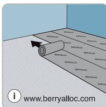
We recommend to install your laminate with a BerryAlloc underlay that suits your situation: reduce footfall noise, floor heating compatible,....
