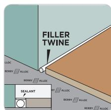
**STEP 1:** Put a **BerryAlloc Fillertwine** in the expansion gap. The fillertwine allows the laminate to expand/shrink. Also use a fillertwine in the expansion gap under floor profiles such as T-profiles, reducers,...
