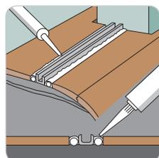
With floor profiles, use sealant on top of the **fillertwine** before you install the profile, to avoid water contact with the side and base of the laminate.
