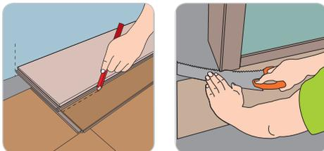
To install the last row, position a panel exactly on top of the previous row. Place another panel upside down up to the wall and mark the panel underneath. Cut the marked panel to size and fit in place. This method should be repeated for each panel until the last row is complete.
