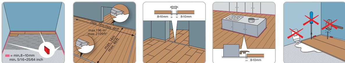
BerryAlloc laminate should be installed as floating flooring which means that the floor should be able to move:
