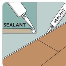
**STEP 2:** Fill the expansion gap with **Hydro+ Sealant**. The sealant should touch the wall and the laminate and be applied in a way that it completely closes the gap.
