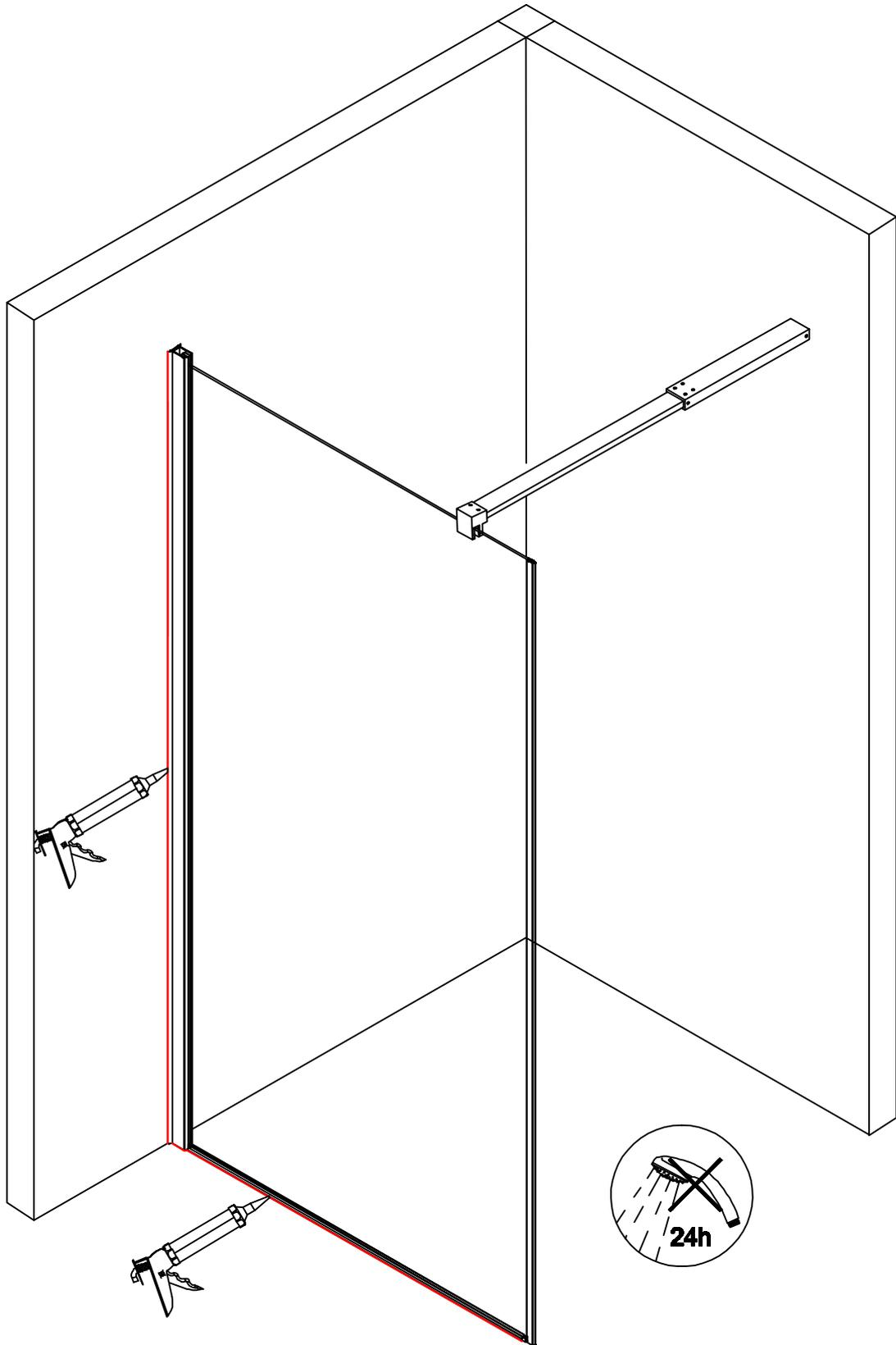
Before the final set up of this shower enclosure, check its watertightness.
