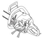
IMPORTANT! In order to maintain operation of the centrifugal cleaning system it must be regularly maintained. Clean the air intake to the starter, the fins on the flywheel, the space around the flywheel, inlet pipe and carburettor compartment.
