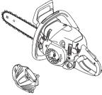
Pull out the cord approx. 30 cm and hook it into the notch in the rim of the pulley. Release the recoil spring by letting the pulley rotate slowly backwards.
